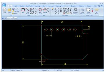
FastCAM® is a system built specifically for the high speed production of line drawings. CNC needs every line, arc or entity to be precise, clean connected geometry.
